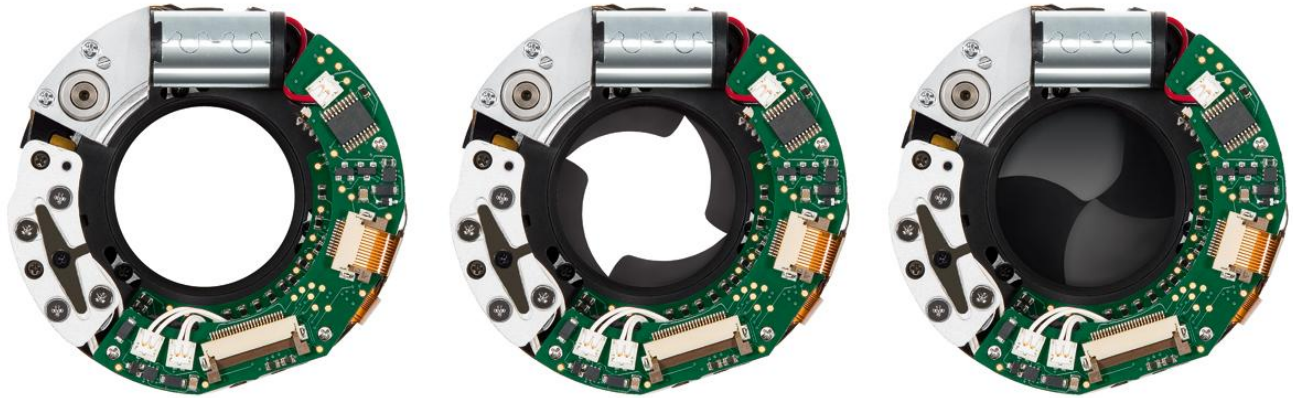
Figure 2: The central shutter generates no vibration and is very fast. The geared DC motor is used for tensioning three springs that store the energy for the central shutter with a bespoke gearhead for small space envelope.
