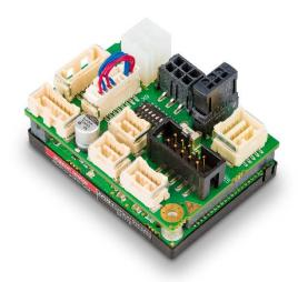
The new positioning controllers EPOS4
